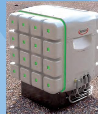
Working with Redox Power Systems LLC, center researchers are developing fuel cell technology that can provide safe, reliable, continuous electricity on site at about one-tenth the cost and size, and at 10 times the power density of current commercial fuel cells.
